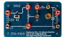
EX10 Measure the VA characteristic curve of small bulb by voltage-tapping approach
